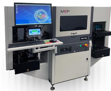
For line integration the 900 series uses SECS/GEM, e-Maps, AutoData SQL integration and ELSRs to provide accurate manufacturing data.
